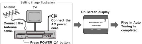
All broadcasting stations that can be received in the area are automatically tuned and stored in memory.
