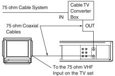
The cable hook-up shown at the bottom left allows VCR-TV functions except for viewing one channel while recording another.
